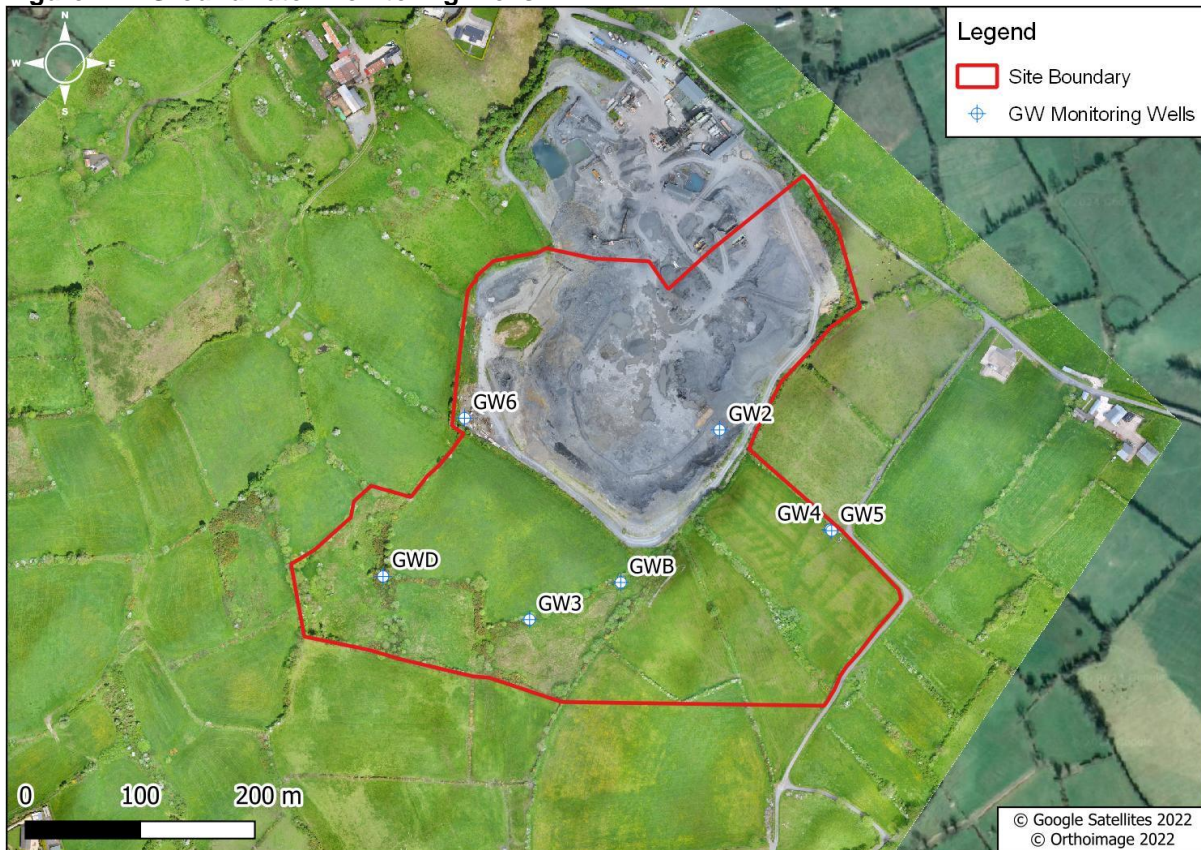
Figure 7-2: Groundwater Monitoring Wells
